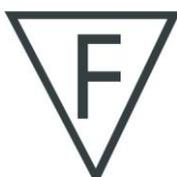
**THIS SYMBOL MEANS "SUITABLE FOR MOUNTING ON NORMALLY FLAMMABLE SURFACES"**
