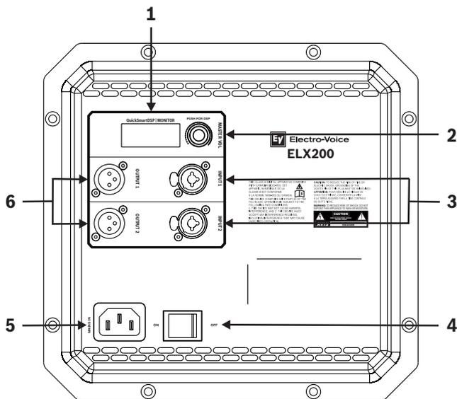
1. **LCD** - DSP control and monitoring interface.
