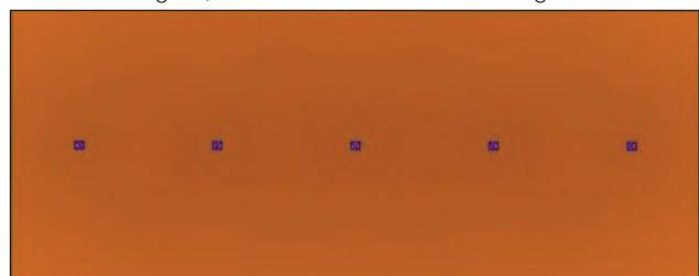
Direct sound at 1kHz obtained with 6" ceiling loudspeakers spaced by 5m, installation height 5,5m: attenuation of -3dB on the edges.
