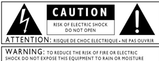
These symbols are internationally accepted symbols that warn of potential hazards with electrical products. The lightning flash means that there are dangerous voltages present within the unit. The exclamation point indicates that it is necessary for the user to refer to the owner's manual.
