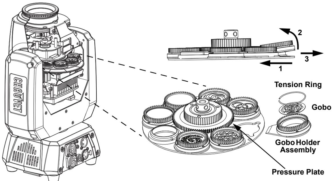
5. Separate the gobo holder assembly from the gobo wheel by pushing it forward and up. Be careful not to push the gobo out of the gobo plate.
