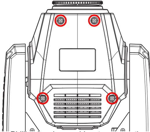
3. Remove 4 screws with a Phillips-head screwdriver to remove the cover.
