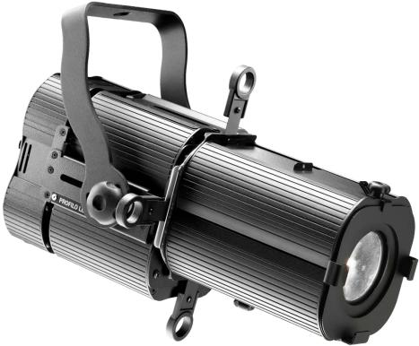
LINEARLY TUNABLE WHITE COLOR TEMPERATURE (2700K – 6000K) INTERNAL 4-SHUTTER SHAPING SYSTEM FLICKER FREE ADJUSTABLE ZOOM 20° - 36° NOISELESS DMX CONTROL EASY MAINTENANCE LONG LIFE LED (50,000 HOURS)
