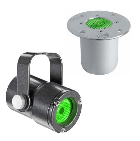
MINI FOCUS FC is a very compact IP65 LED projector available with an orientable bracket or with a recessed flange (MINI FOCUS R FC). The unit is fitted with one high power RGBW LED. The unit is suitable for shopping centers, restaurants, museums, clubs and any application where high quality color mixing and extracompactness are required.
