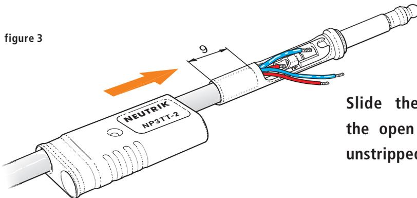
Slide the prepared end of the cable into the open end of the plug, so that 9 mm of unstripped cable rests inside the plug.
