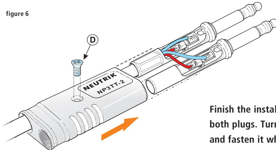
Finish the installation sliding the housing over both plugs. Turn the screw **(D)** into the housing and fasten it while fixing both connectors to the housing.
