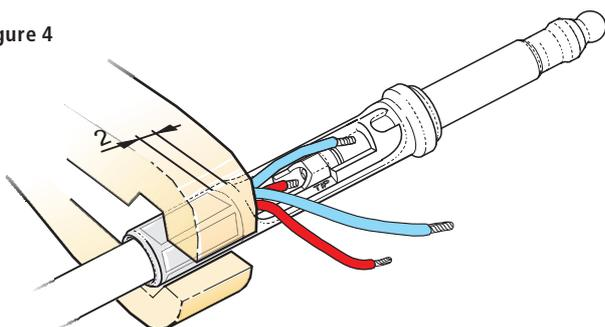
Next crimp the end of the plug with a standard 6.35 mm hexagonal crimping tool (RG 58).
