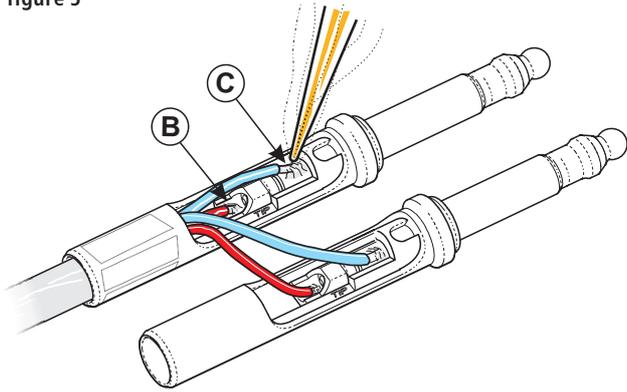
Heat the tip terminal labelled **(B)** with a soldering bit, then position the shorter wire (T1) on the heated terminal and allow solder to melt affixing the wire to the terminal. Repeat the process with the ring terminal labelled **(C)** in figure 5 with the longer wire (R1). Connect the second plug correspondingly.
