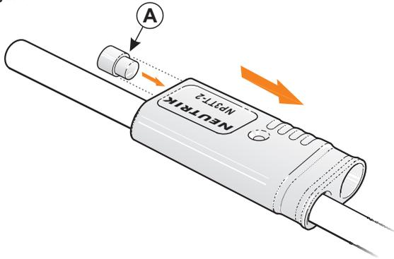
First slide the housing onto the cable and insert the sealing cap **A** into the other hole.
