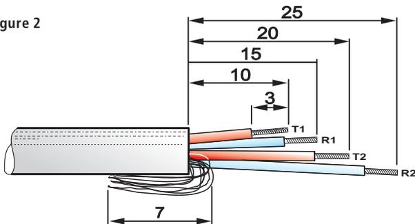
Prepare the cable by stripping 25 mm of the jacket.
