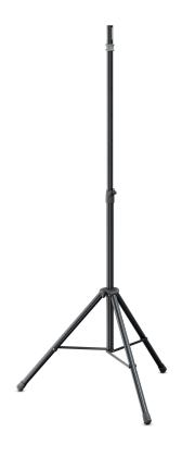
A patented expanding mandrel with quick-release fastener ensures a tight fit of the speaker cabinet. The plastic expansion splints ensure a vibration-free connection between the speaker cabinet and the tube. The height of the steel stand ranges from 1,417 to 2,117 mm, is fixed with a safety hook and secured by a clamping screw for a vibration-free and firm fit. Other features include a pull-out guard for the extension tube, an integrated shock absorber and durable powder coating.
