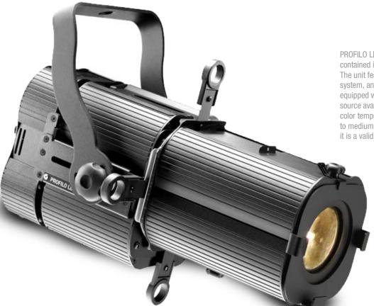
PROFILO LED 80 is a LED-based profile spot contained in a strong and lightweight housing. The unit features an internal four-shutter shaping system, and a 20° to 36° linear zoom. The unit is equipped with a high efficiency 80 W white LED source available with 3000 K, 4000 K, or 5000 K color temperature. The unit is suitable for small to medium TV studios, theatres or museums and it is a valid alternative to conventional light.
