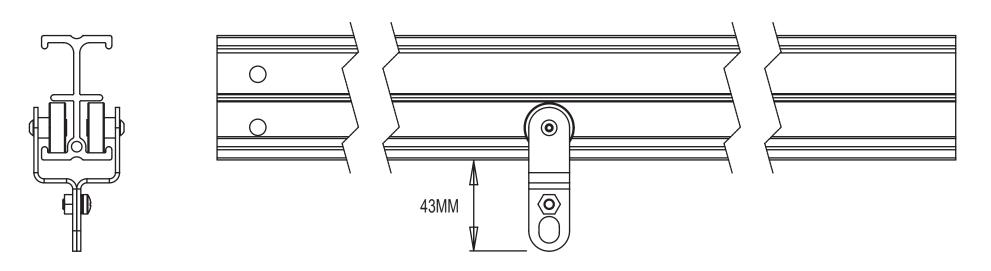
SWL = 6 KG PER CARRIAGE RECOMMENDED SPACING 300MM
