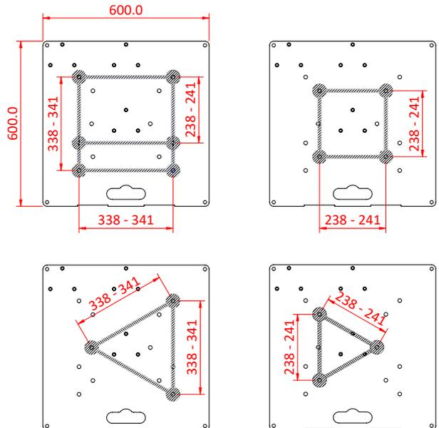
TANK TRAP BASE USED AS TRUSS MOUNTING PLATE
