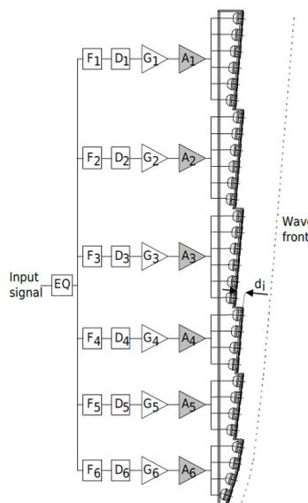
StepArray columns implement the DGRC line-array principle (Digital and Geometric Radiation control) which is a synthesis of geometric and electronic arrays patented by Active audio.
