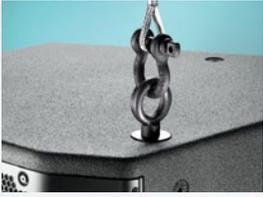
**Suspension Points** | Permanently mounting the PRX400 is easily managed via twelve built-in M10 suspension points constructed from 14 gauge steel. They have been tested with a yield-strength of 1000 pounds each ensuring a safe and secure mount.
