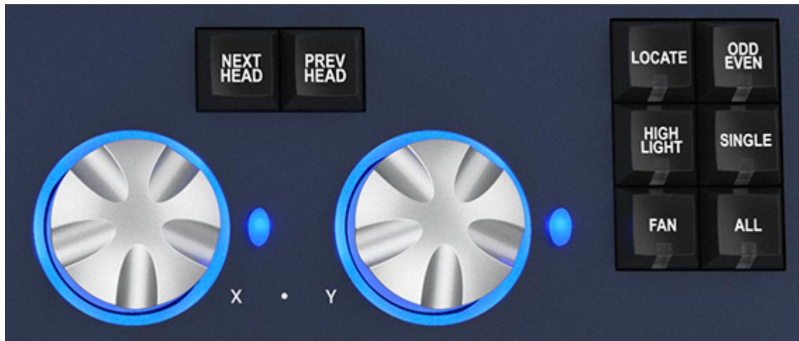
The NEXT HEAD and PREV HEAD buttons are used to select an individual head to modify.
