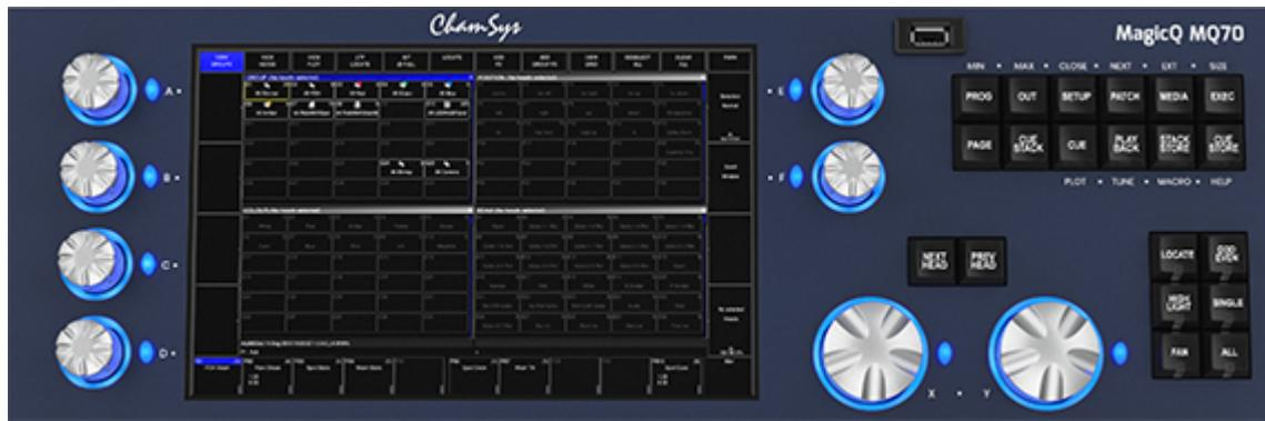
The function of the rotary encoders changes according to the active window with the current function being displayed adjacent to the encoder.
