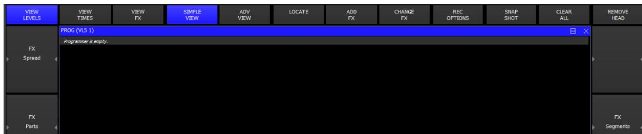
In the Channel Times and Channel View windows you have a choice of a Simple View or an Advanced View. The Simple View is sufficient for most programming – it enables modifications of fade times on a per attribute type basis and modifications of each programmed FX. The Advanced View enables fade times and FX parameters to be set up on a per channel basis.
