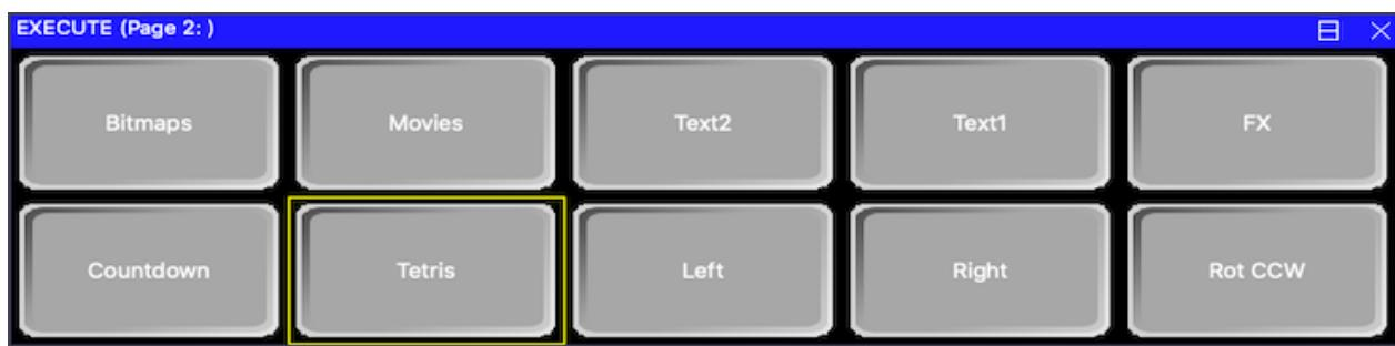
Buttons can also be set as solo buttons (also known as radio buttons) so that a group of buttons programmed as Cues or Cue Stacks can be set so that only one of the group is active at a time. Use soft button E to select "Solo".
