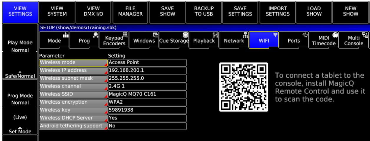
*Wireless mode* needs to be set to "Access Point" or "Access Point (Hidden SSID)".
