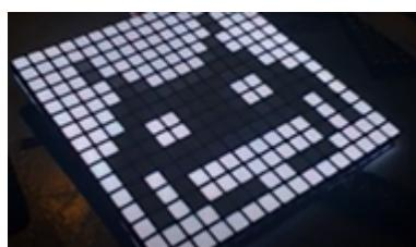
MagicQ enables LED heads to be used in their "high resolution" mode enabling individual control of each LED pixel rather than the restricted modes where Lighting Designers are reliant on the same old in built effects that everyone has seen many times.
