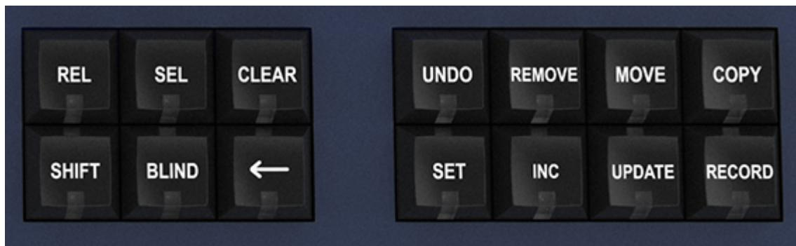
The Editor buttons are used to modify program data. The 8 buttons on the right hand side are the action buttons which are used to modify show data. The action buttons are UNDO, REMOVE, MOVE, COPY, SET, INCLUDE, UPDATE, and RECORD.
