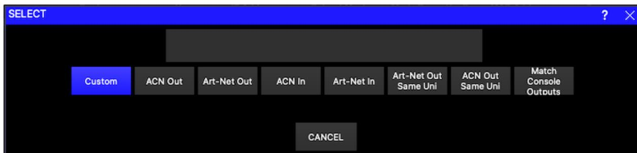
The profiles act as a starting point – once a starting profile has been chosen, the detailed configuration can all be set individually for each port by changing to the VIEW PORTS view.
