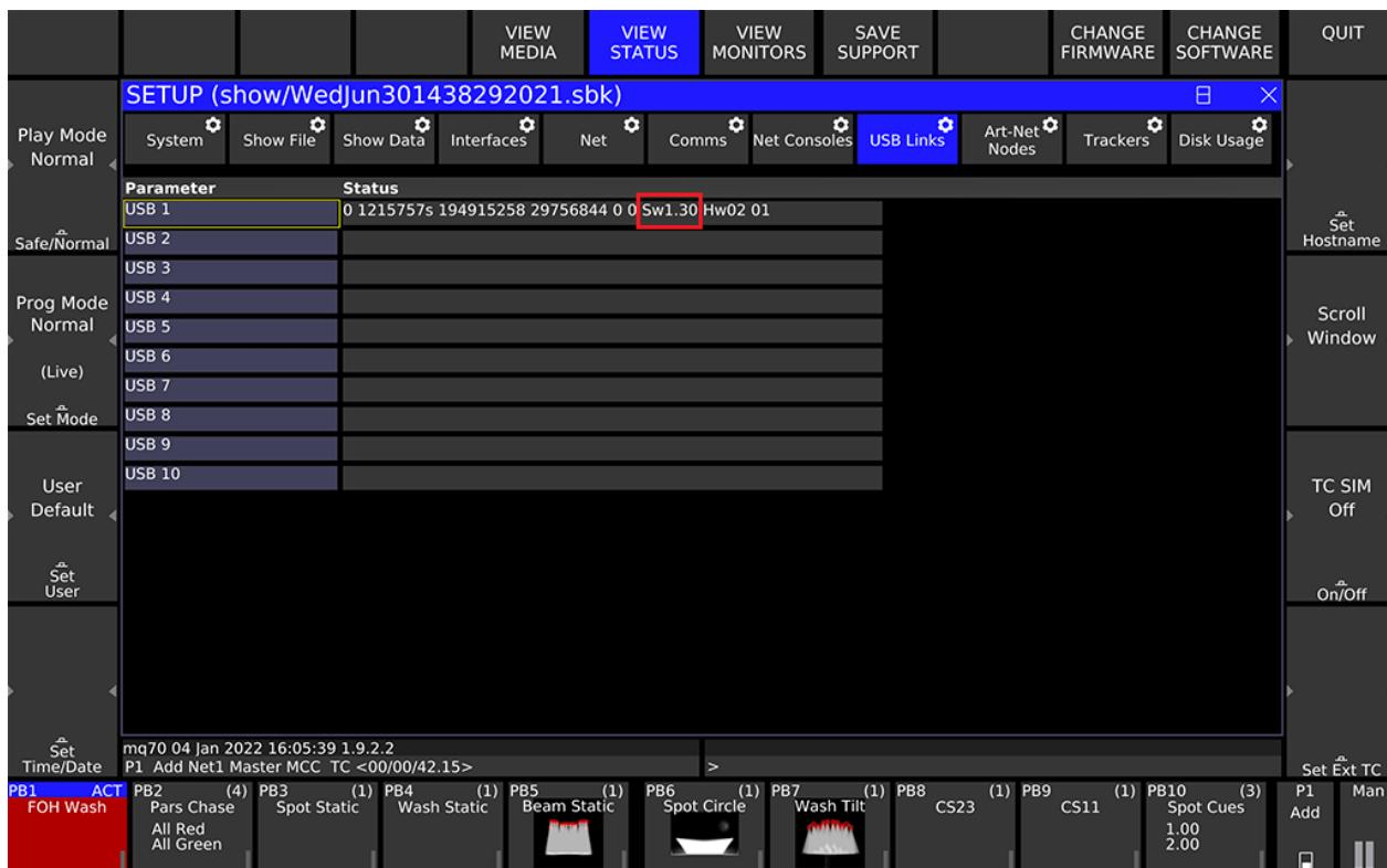
Some MagicQ installers will not include every version of the CH346 firmware, however a higher version will include fixes and features of a lower version. i.e. CH346 V1.25 will include all fixes and features of the lower versions.
