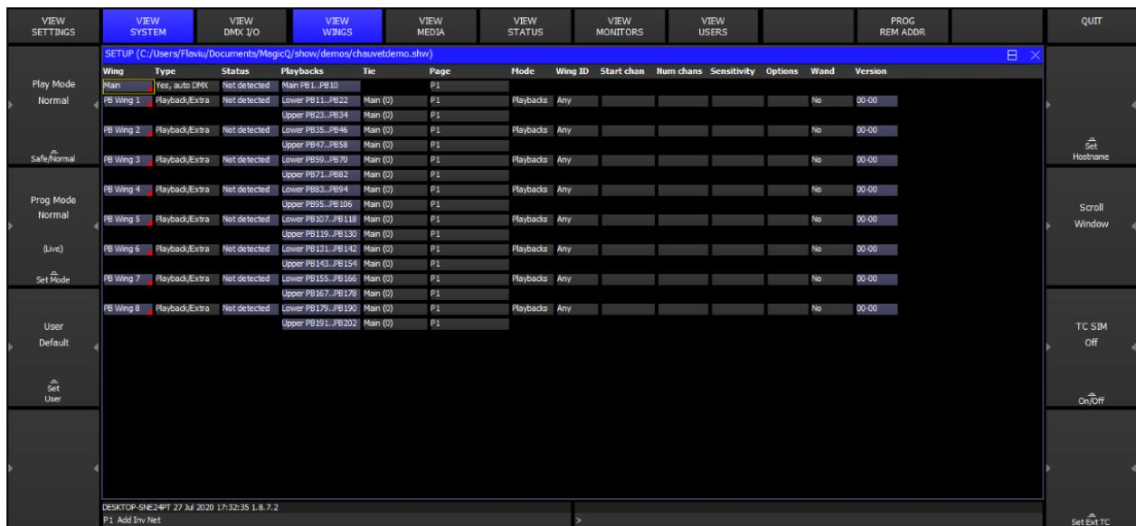
To enable the Scene Setter in MagicQ software, set one of the Wings in Setup, View System, Wings to "Remote Panels".
