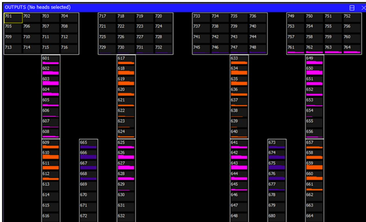
In the Outputs Window, select View Plan. Then select View Grid and View Head Nos. Press Grid Size and enter a matrix size for your lighting rig – e.g. 30/20 gives a 30 column by 20 row grid.
