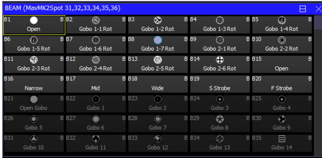
For indexed attributes such as colour wheels and gobo wheels, the button associated with each encoder can be used to bump the attribute value to the next range. Pressing SHIFT and the button bumps back to the previous range.
