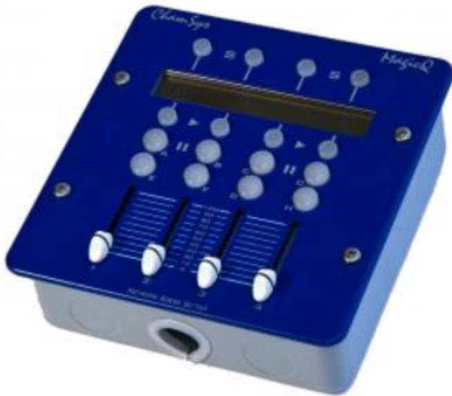
The MagicQ Scene Setter enables control of MagicQ from a remote location using a fixed network connection. The Scene Setter has 4 playback faders and 12 playback buttons, and can be mapped to the wing playbacks on a MagicQ system. An LCD screen shows the legends for the playbacks.
