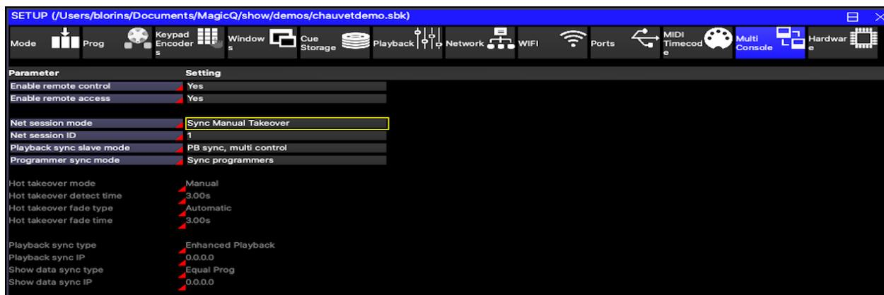
The first console to start becomes the Master. In Setup, View DMX I/O, Take Control and Release Control can be used to swap which console is the Master at any time. If you use Release Control, then you will need to also press Take Control on the other console.
