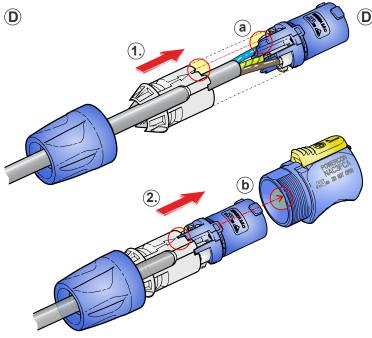
D Slide the insert and the chuck (1) into the housing (2).
