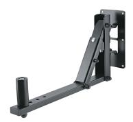
Robust speaker wall mount for speaker cabinets with flange socket receptacle. Max. recommended load 25 kg. Thanks to the appropriate design, the bracket is almost completely concealed by the speaker. The speaker distance to the wall is selectable in 4 steps. The swivel range is infinitely adjustable, and the tilt angle can be fixed in 6 steps up to max. 30 °.
