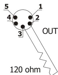
PLACE A 120 OHM RESISTOR BETWEEN PIN 2 AND 3 OF A MALE XRL CONNECTOR AND PLUG IT INTO THE DMX OUT PANEL CONNECTOR OF THE LAST UNIT CONNECTED TO THE DMX LINE
