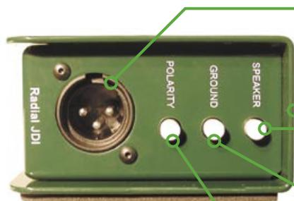
**XLR** balanced 600Ω mic-level output for runs to 1000 feet without appreciable noise.
