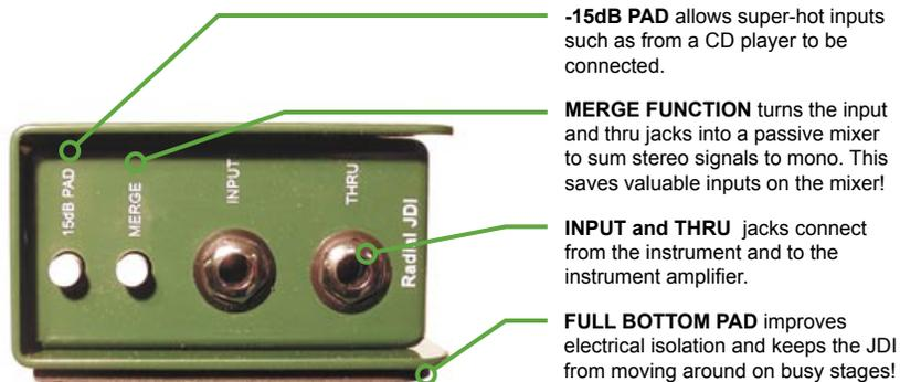
**-15dB PAD** allows super-hot inputs such as from a CD player to be connected.
