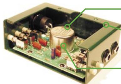
**JENSEN** nickel core transformer for distortion-free signal transfer and 100% isolation.
