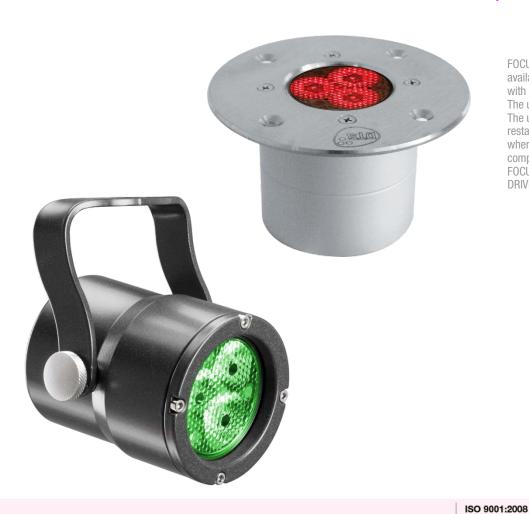
FOCUS FC is a very compact IP65 LED projector available either with an orientable bracket or with a recessed flange (FOCUS R FC). The unit is fitted with 3 high power RGBW LEDs. The unit is suitable for shopping centers, restaurants, museums, clubs and any application where high quality color mixing and great compactness are required. FOCUS FC must be powered by an external PSU: DRIVENET 416, 832, or 1664.
