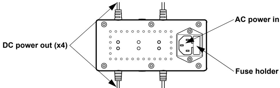
The Freedom Q1N Multi-Charger is an auto-ranging power supply, and it can work with an input voltage range of 100 to 240 VAC, 50/60 Hz. To determine the product's power requirements (circuit breaker, power outlet, and wiring), use the current value listed on the label affixed to the product's back panel, or refer to the product's specifications chart. The listed current rating indicates the product's average current draw under normal conditions.
