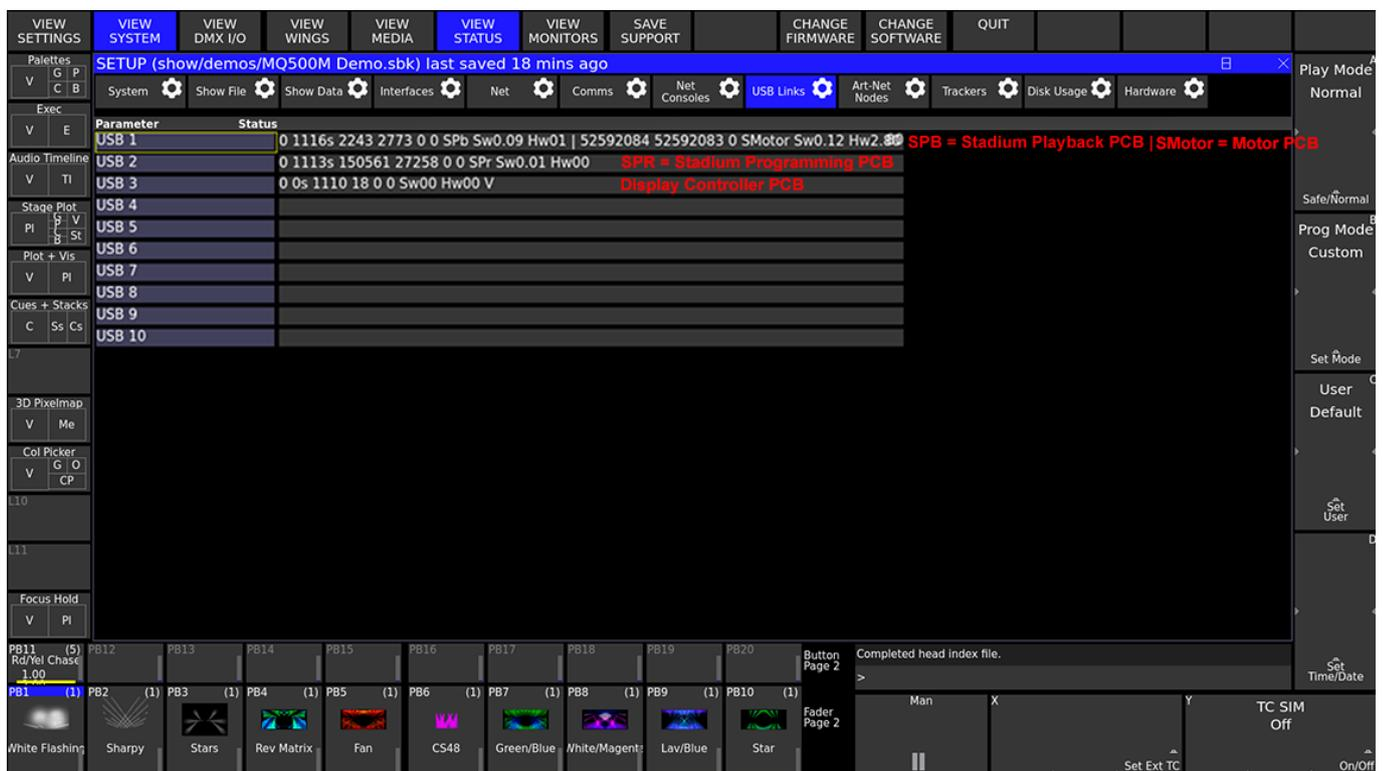
To check the version of firmware in use go to Setup, View System, View Status and select the Hardware tab. For each panel/board it shows current version, available highest firmware version and current update status.
