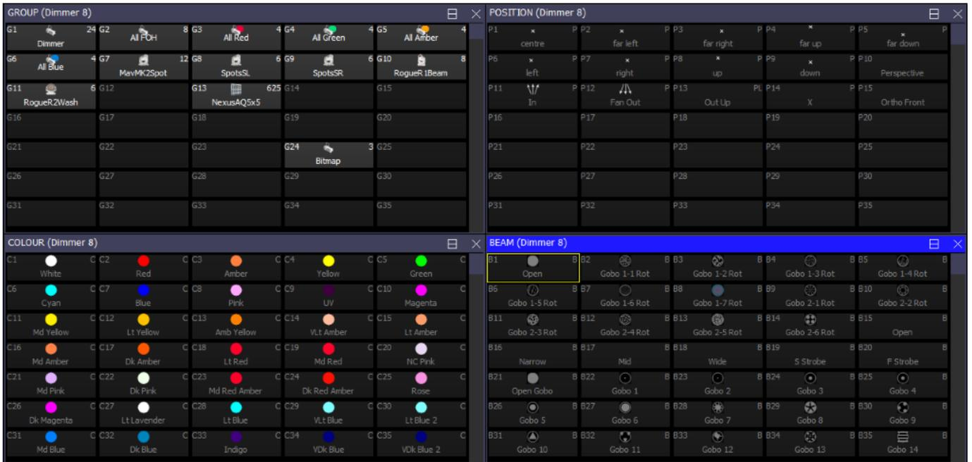
The highlighted window enables controls the soft buttons and rotary encoders. In each of the Windows the X and Y encoders control the most important attributes – Pan and Tilt in Position Window, Col Wheel 1 and Col Wheel 2 in the Colour Window and Gobo Wheel 1 and Gobo Wheel 2 in the Beam Window. In the Beam Window there are more than eight attributes to be controlled – these are accessed using multiple pages of encoders – by pressing the NEXT PAGE soft button.
