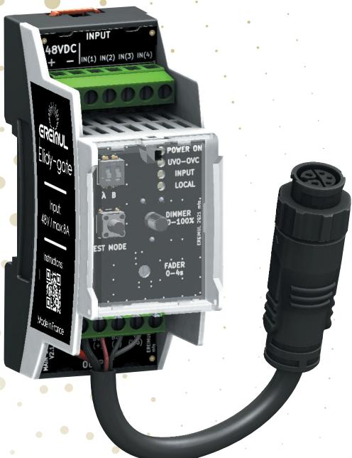
The “PIXELIDY GATE” is the “bridgehead” of the Pixelidy system. As well as merging the 48V power supply and the DMX signal onto a single output, it provides electrical protection and isolates the signal from all the peripherals connected downstream.
