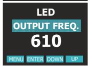
**OUTPUT FREQUENCY** Range = 610 Hz - 20 KHzDefault = 610 Hz
