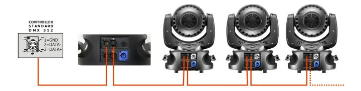
For Installations where long distance DMX cable connections are needed, we suggest to use a DMX terminator.
