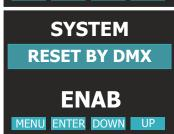
RESET BY DMX Enable: Motors reset enabled
