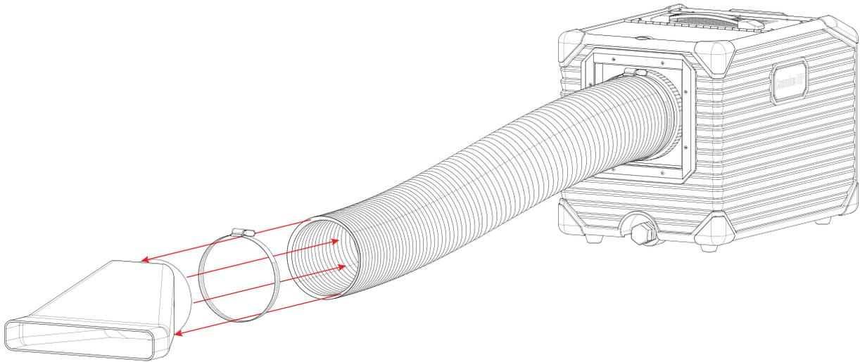
5. Ensuring the hose clamp is over both the hose and the floor nozzle, turn the wingnut clockwise until the hose is secured to the floor nozzle.
