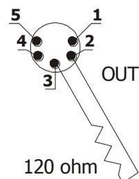
PLACE A 120 OHM RESISTOR BETWEEN PIN 2 AND 3 OF A MALE XLR CONNECTOR AND PLUG IT INTO THE DMX OUT PANEL CONNECTOR OF THE LAST UNIT CONNECTED TO THE DMX LINE
