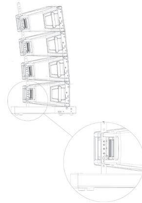
5) The bottom box in a stacked array can be tilted to obtain proper coverage patterns (from +7,5° to -7,5°). Reverse and connect the 1 rear stacking bar bracket to the first enclosure using the hole for the proper angle and quick lock pins.
