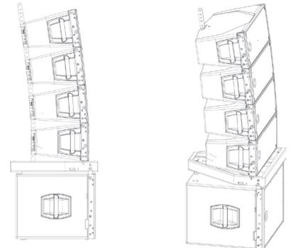
2) The stacking bar adds a fixed amount of up or down tilt to ground-stacked HDL modules, with additional 15 degrees of adjustment possible (from  $+7,5^\circ$  to  $-7,5^\circ$ ).
