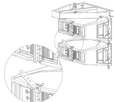
7) Connect all the other cabinets following the same procedure and connecting a single cabinet each time.
