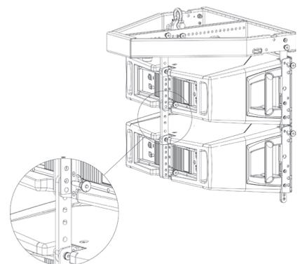
HDL allow users to choose from different face-to-face angle adjustments to create arrays with varying curvature. Thus, designers can create arrays custom-tailored to each venue's profile.
