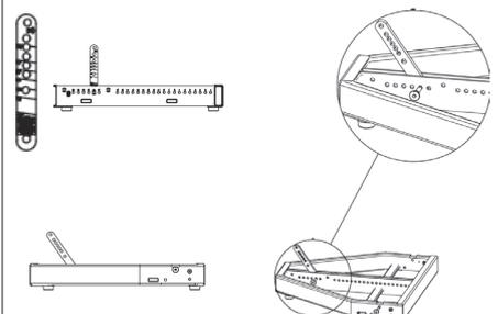
3) Connect front bracket of the first HDL cabinet using 2 quick lock pins.
