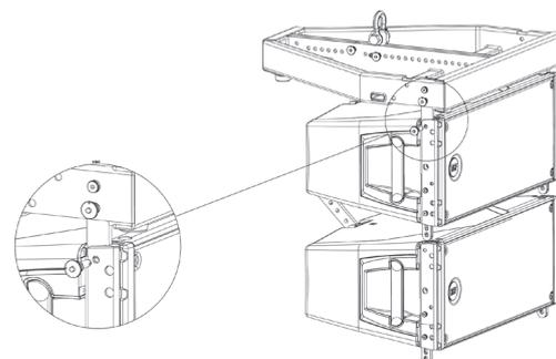
4) Reverse and connect the 1 rear bracket to the fly-bar using 2 quick lock pins. The first HDL has to be fixed always starting at 0° with respect of the frame. No other angles are allowed.
