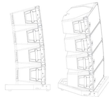
6) It is possible to stack HDL speakers on the ground using its own fly bar as shown in the pictures.
