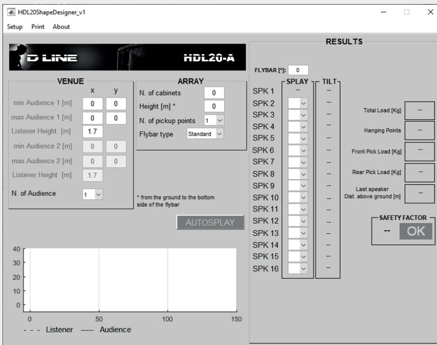
Once the design (number of elements and vertical splay angles) has been designed using Shape Designer software, you can effectively optimise the array depending on the environment and the application by driving it using different DSP presets stored onboard. Typically arrays are divided in two or three zones depending the design and size of the array.
