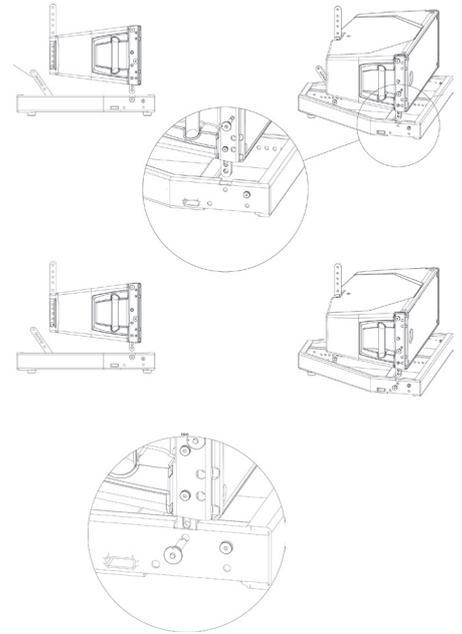
4) The baffle of the bottom box in a stacked array does not necessarily have to be parallel to the stage or the array frame. It can be tilted up or downward if desired. In this way arced arrays can be readily created from a ground stack position.
