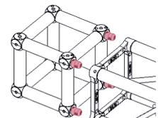
**CONNECTING TO THE TRUSS** Connecting Dado to a truss is straightforward and intuitive. You will need both the conical pins and safety split-pins. **NOTE:** the conical pins must be hammered hard into the connectors.
