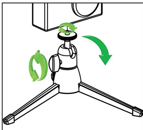
Screw the equipment onto the stand. If necessary, the equipment can be locked in place with the help of the knurled disc. To adjust the direction or the angular position, hold the screwed-on equipment and loosen the clamping screw. Set the desired position and retighten clamp. Dismantling is carried out in reverse order.
