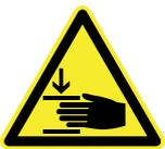
***!When adjusting the position, there is a crushing risk between the components!***
