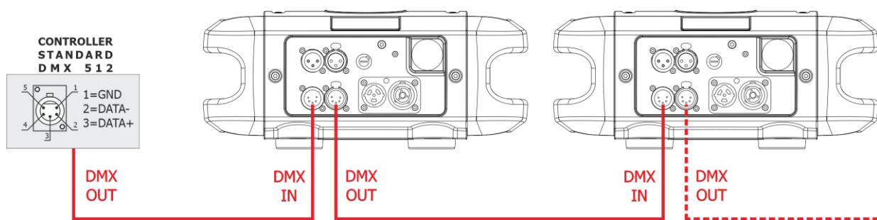
For installations where long distance DMX cable connections are needed, we suggest to use a DMX terminator.
