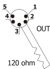
PLACE A 120 OHM RESISTOR BETWEEN PIN 2 AND 3 OF A MALE XRL CONNECTOR AND PLUG IT INTO THE DMX OUT PANEL CONNECTOR OF THE LAST UNIT CONNECTED TO THE DMX LINE
