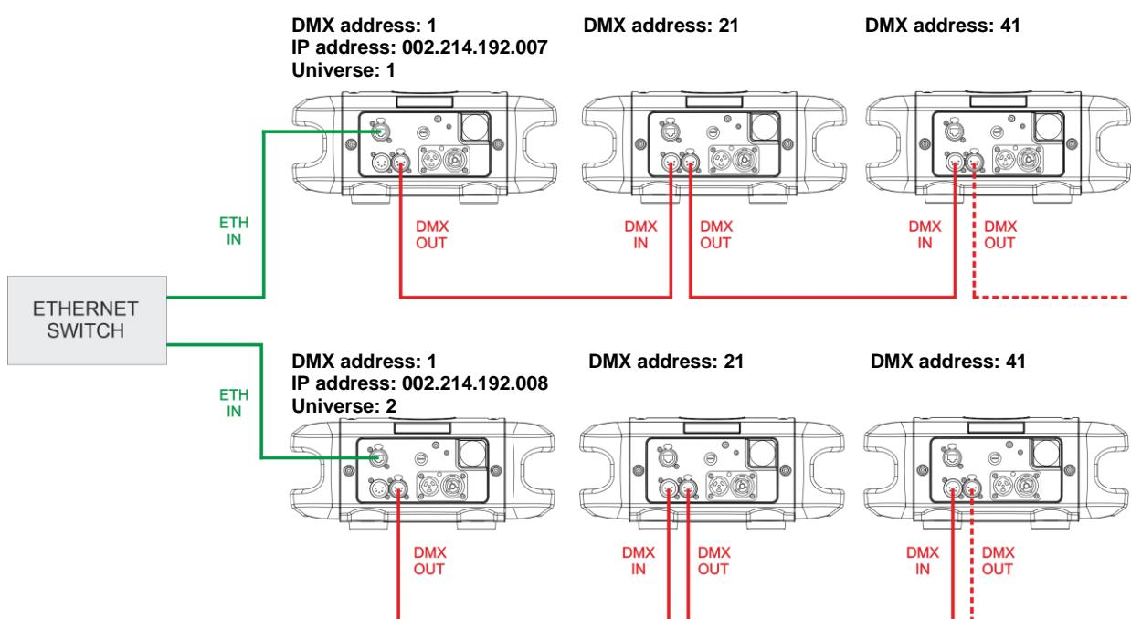
For installations where long distance DMX cable connections are needed, we suggest to use a DMX terminator.
