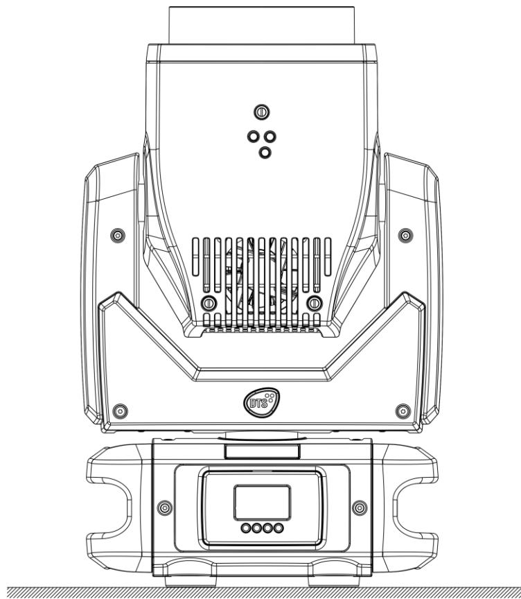
For ceiling mounted installations, we recommend the use of appropriate clamps to fix the unit to the mounting surface.
