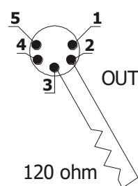
PLACE A 120 OHM RESISTOR BETWEEN PIN 2 AND 3 OF A MALE XRL CONNECTOR AND PLUG IT INTO THE DMX OUT PANEL CONNECTOR OF THE LAST UNIT CONNECTED TO THE DMX LINE
