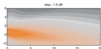
Step Array SA100P vertical directivity: sound level for the speech octaves (500Hz-1kHz-2kHz) in the vertical median plane.
