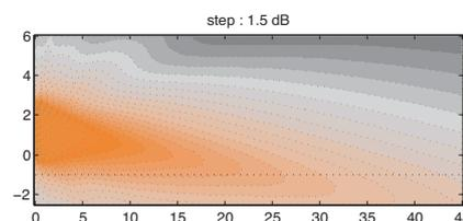
Step Array SA250P vertical directivity: sound level for the speech octaves (500Hz-1kHz-2kHz) in the vertical median plane.
