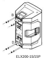
4. Using the four screws you removed from the bottom handle, attach the **lower mount (D)** to a 12-inch or 15-inch loudspeaker where the bottom handle was located in the up position.
