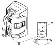
5. Position the **loudspeaker** to the desired angle.
