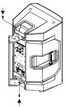
Tighten the two M6 screws (supplied) sufficiently so the loudspeaker does not rotate. The loudspeaker is set to the desired angle.
