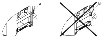
Figure 1.1: Eyebolt shown with and without washer; (left Correct A: Washer used; right Incorrect B: No washer used)
