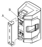
4. Ensuring the lower U-Bracket pivot pin (A) is securely placed in the notch; guide the **lower mount with hook (B)** into position.
