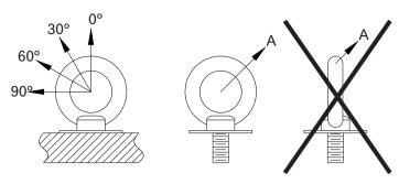
Figure 2.2: Load angles and suspension point (Left load angles, center Correct and right Incorrect); A: Direction of load
