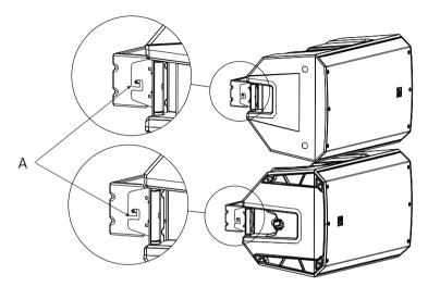
Figure 2.1: Horizontal mounting slot orientation with the lower mount slot opening on the bottom (A) To attach the mounts to a loudspeaker, do the following:
