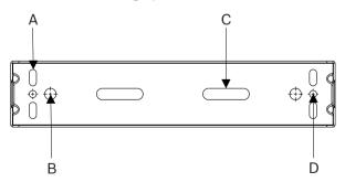
A: For wall mounting with bolts (3/8" or M10 bolts) OR pole/truss mounting with U-bolts (2" or M10 U-bolt) (4 PLS)
