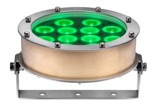
HELIOS BRONZE 12 FC is an IP 68 underwater projector with RGBW LEDs. The unit is fitted with an adjustable bracket or a round flange (HELIOS BRONZE 12 R FC) for recessed installation. The unit features a reinforced structure that makes this product reliable for long-term use. The unit is available with different optics. HELIOS BRONZE 12 FC is the brightest projector in its range, and it is suitable for fountains and other water features.
