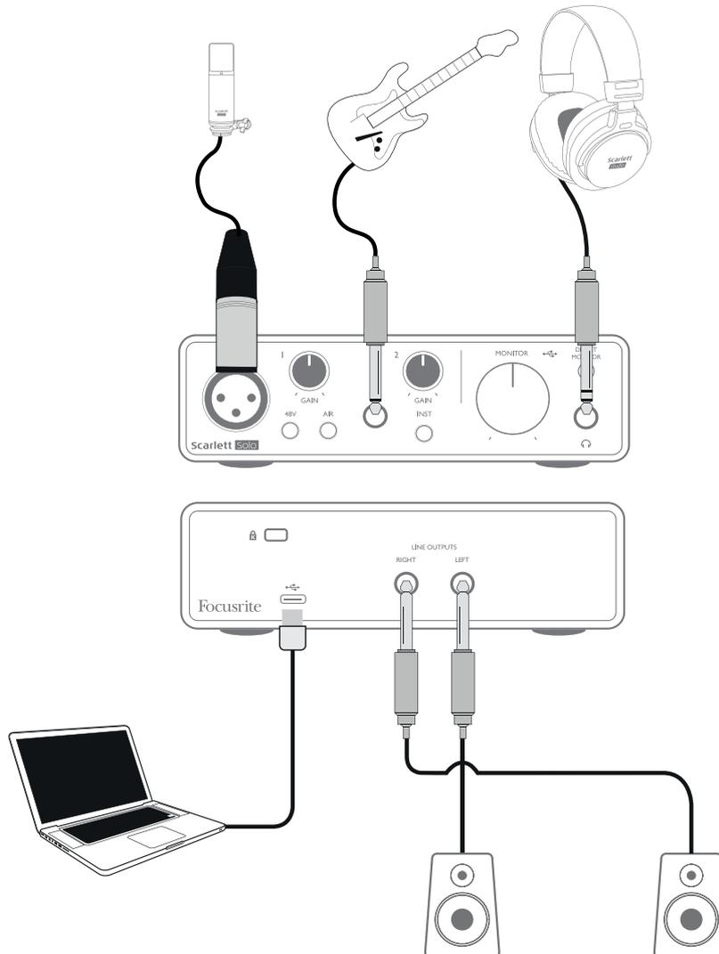
This setup illustrates a typical configuration for recording using DAW software on your Mac or PC. In this case, you would record vocals through Input 1 and guitar through Input 2 into your recording application, while monitoring the playback via headphones.
