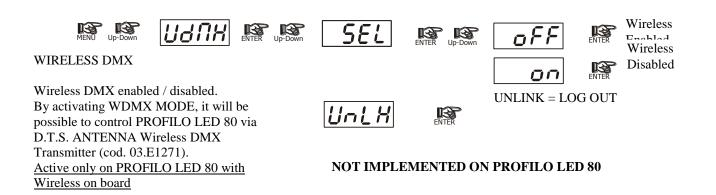
Logging on PROFILO LED 80 (WIRELESS DMX must be enabled on PROFILO LED 80 unit)
