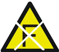
**THIS SYMBOL MEANS “DO NOT PLACE THE UNIT ON INFLAMMABLE SURFACES”**
