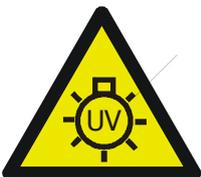
**THIS SYMBOL MEANS “RADIATION FROM THIS LAMP CAN CAUSE DAMAGE TO EYES AND SKIN”**
