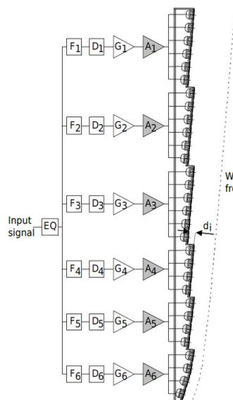
StepArray columns implement the DGRC line-array principle (Digital and Geometric Radiation control) which is a synthesis of geometric and electronic arrays patented by Active audio.
