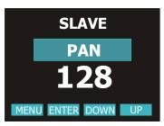
The SLAVE unit receive DMX signal from the MASTER unit. By setting all the SLAVE units connected to the MASTER, to DMX address 1, them will be synchronized with the Master unit following the chase selected on it, but running their own Pan&Tilt and Zoom position.
