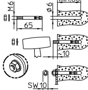
BRICK WALL: frame fixings  $\varnothing$  8 x 80 mm with wood screws M6 x 85 mm; pre-drill  $\varnothing$  8 mm / 90 mm deep.
