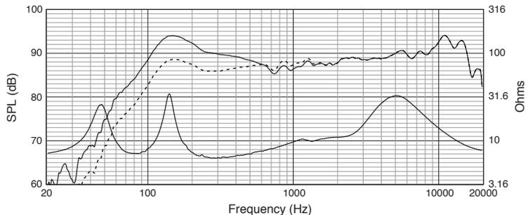
On-axis in half-space (2pi, solid line) and full-space (4pi, dotted line) at thru (8Ω) setting; input impedance (lower solid line)
