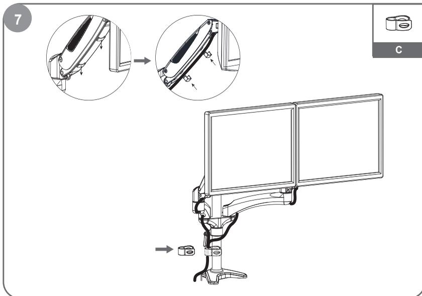
Insert cables into cable covers.
