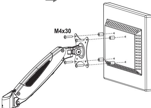
Flush surface installation: Install 4 screws through faceplate to monitor via mounting holes.
