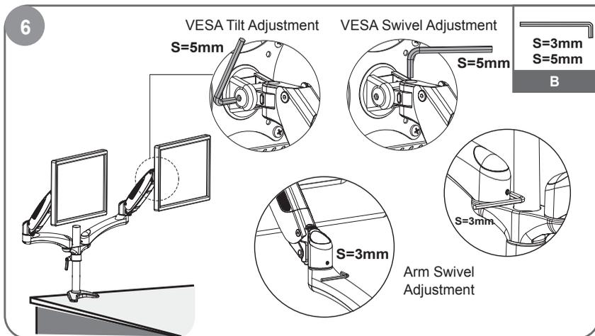
Use a hex wrench to adjust the damp for swiveling. Turn counter-clockwise to reduce damping and clockwise to increase damping.
