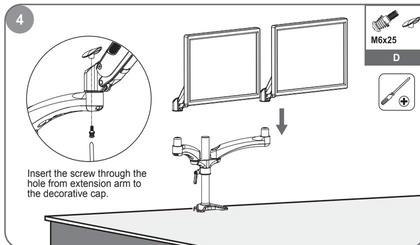
Lift the spring arm along with the monitor and put it on the extension arm.
