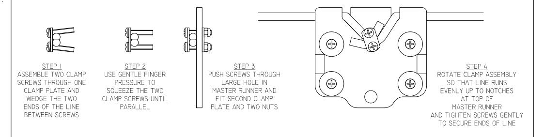
THESE VIEWS SHOW STEP BY STEP PROCEDURE TO ATTACH ENDS OF LINE TO MASTER RUNNER
