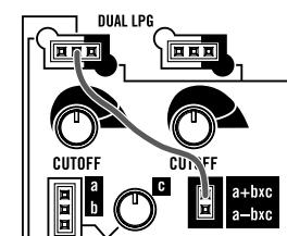
Turn both the LPG's CUTOFF knob and UTILITY's "c" knob all the way up, and you should hear the SOURCE's carrier audio signal. Set the MOD, RATIO, and FOLD knobs to various values and hear how the timbre changes.
