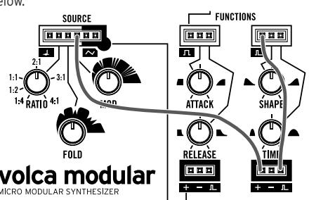
Set the Rise-Fall generator knobs to various values and hear how the timbre is modulated at different speeds and following different curves.
