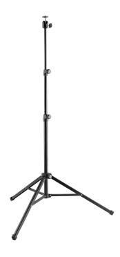
Useful camera tripod for mounting compact cameras, action cameras, web cams, mini-projectors and mobile recorders with a 1/4" connection thread. The ball joint allows the mounted equipment to be rotated 360° and fixed in any position. The tilt-angle is infinitely adjustable up to 90° and the load capacity is designed for equipment up to 1 kg. The height can be freely adjusted from 555 mm to 1355 mm via two extensions. For transport, the tripod folds compactly to save space.
