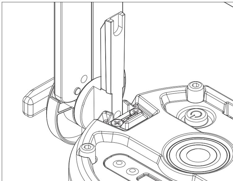
2. Push the yoke downward until the bracket release latches click into place.
