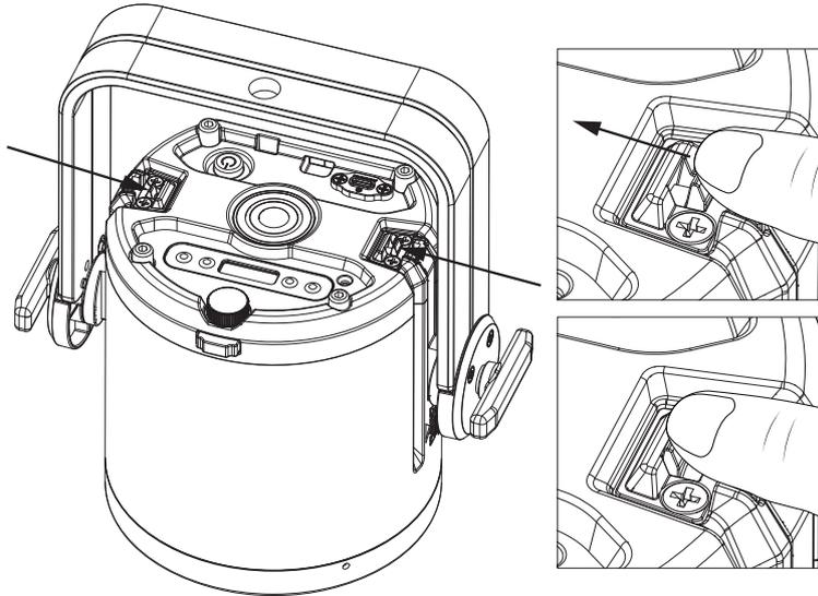
2. While pinching both bracket release latches inward, pull the yoke up and away from the fixture.
