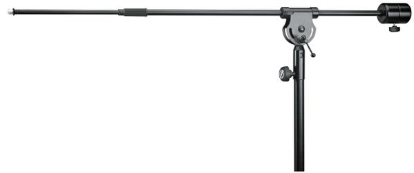
Extendable boom arm with 3/8" or 5/8" microphone thread connection. The sturdy tube combination with diameters of 20 and 15 mm provides a usable extension length of 1,670 mm. A 3 kg counterweight assures the necessary balance. Thanks to the  $\varnothing$  35 mm stand adapter, the boom arm can be combined with common speaker and lighting stands.
