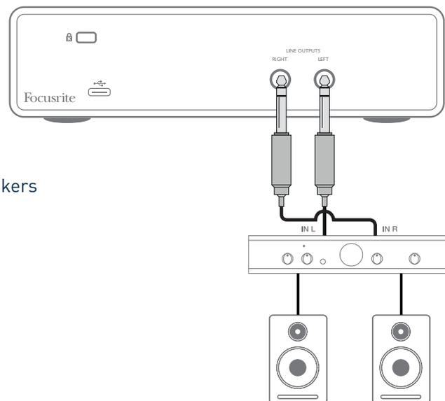
The line outputs are 3-pole (TRS) ¼" (6.35 mm) jack sockets, and are electronically balanced. Typical consumer (Hi-Fi) amplifiers and small powered monitors will have unbalanced inputs, either on phono (RCA) sockets, or via a 3.5 mm 3-pole jack plug intended for direct connection to a computer. In either case, use a suitable connecting cable with jack plugs at one end.
