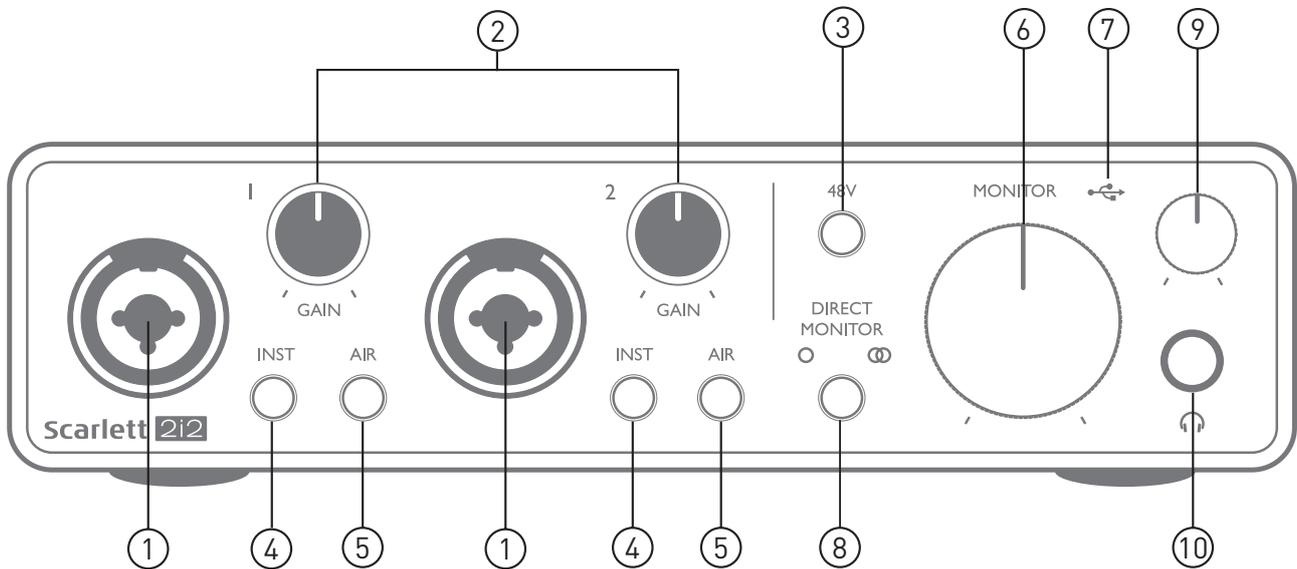
The Front Panel includes the input connectors for Mic, Line and Instrument signals, as well as the input gain and monitoring controls.
