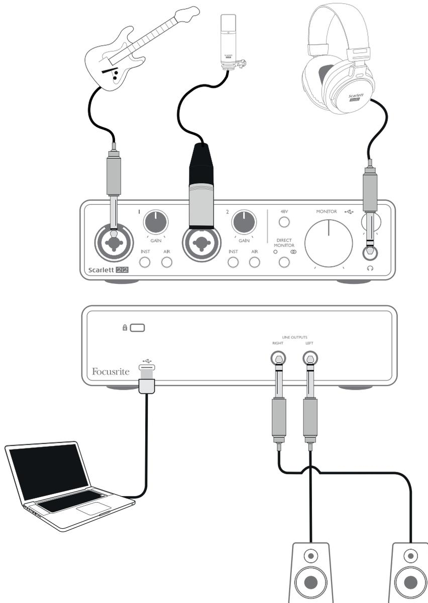
This setup illustrates the most typical configuration for recording with DAW software on your Mac or PC. In this case, you might record guitar through Input 1 and vocals through Input 2 into your DAW, while monitoring the playback from the DAW via headphones (or speakers).
