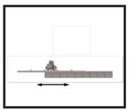
STEP 6: Loosen the lever on the base and push the leg section all the way down to the bottom of the main tube.
