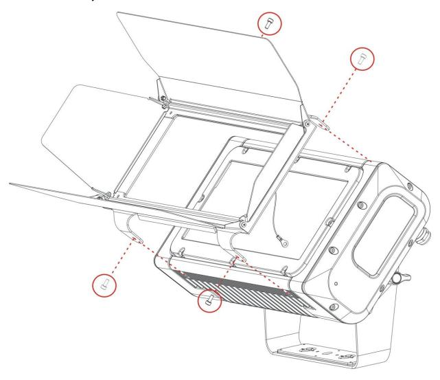
Once installed, fix the safety cable on the side cap by using the marked screw and the washer provided in the box as shown in the picture.
