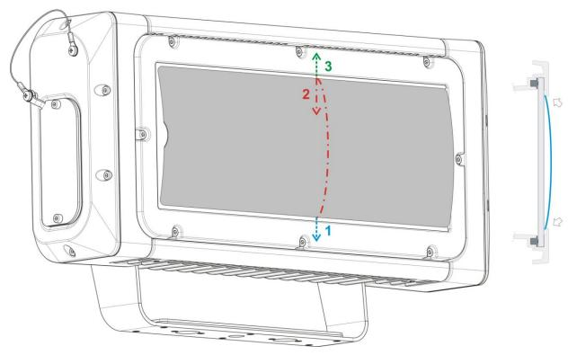
To remove the filter simply lift with a finger the filter on the side with the opening as shown in the picture.
